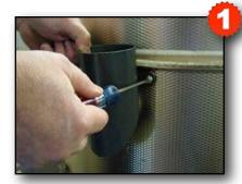
1) Remove existing Nabertherm exhaust stack by removing the two screws holding the stack to the side of the kiln.
