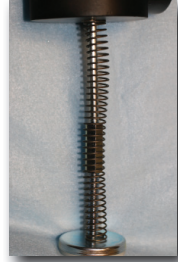
Completed Spring Loaded Pedestal
