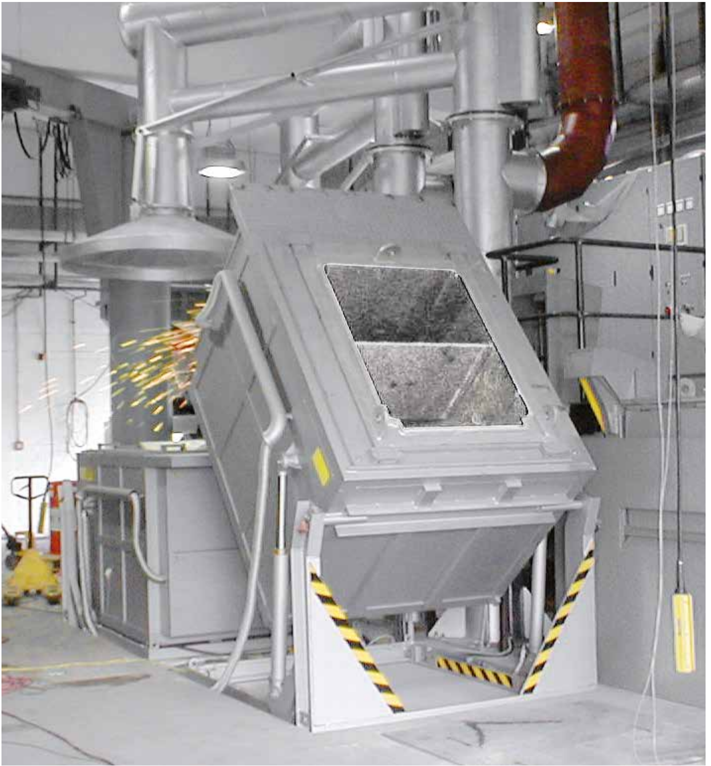
Tilting furnace K 1500/75 S for magnesium with 1500 liters crucible volume
