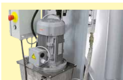
Hydraulic system with flame resistant hydraulic fluid
