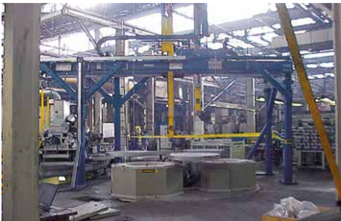
Rotary table system with three bale-out furnaces T 150/11
