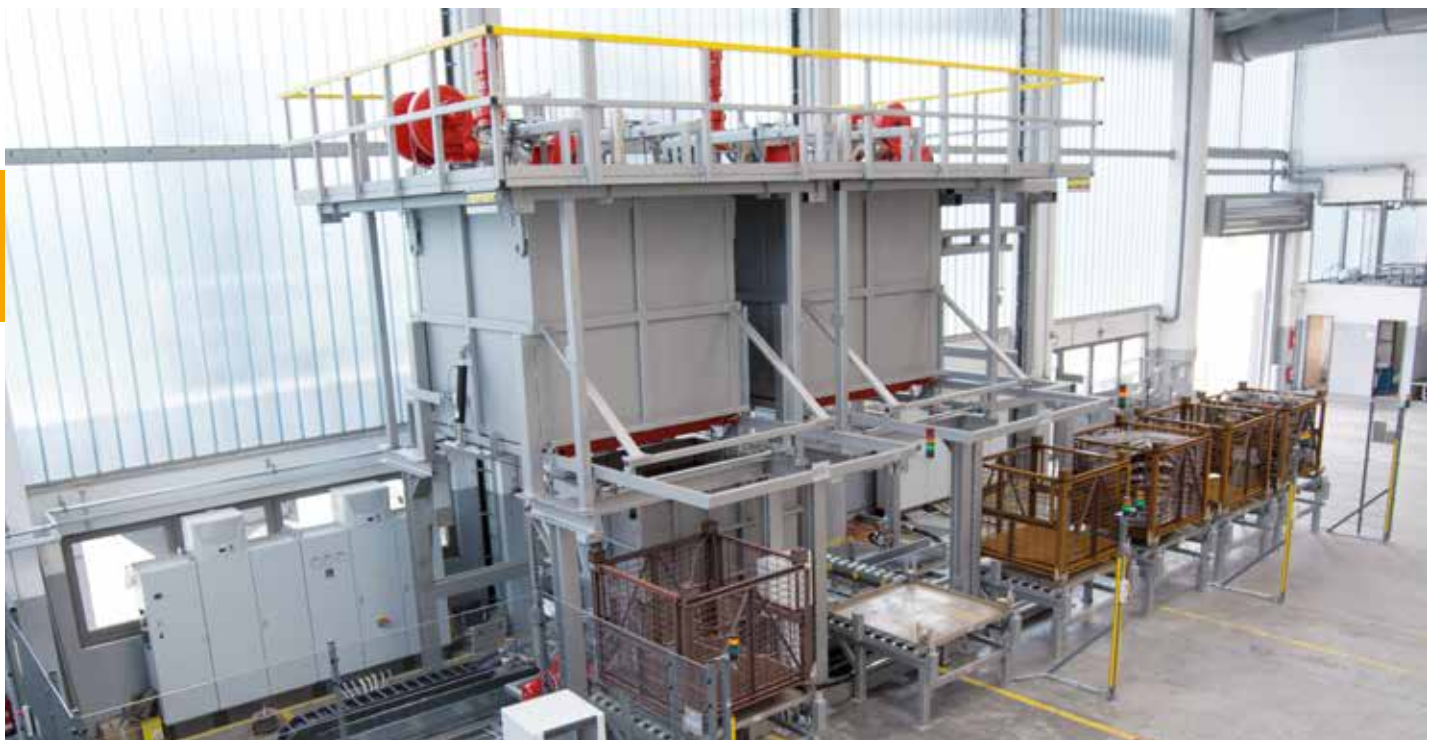
Fully automatic drop-bottom furnace plant, consisting of two drop-bottom furnaces, movable water bath and several loading and unloading positions
