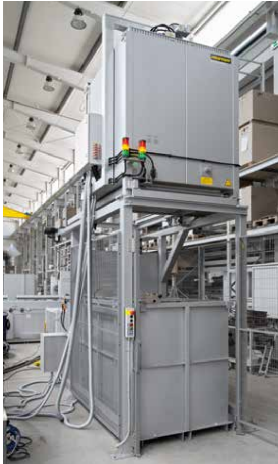
Drop-bottom furnace with fixed quenching bath
