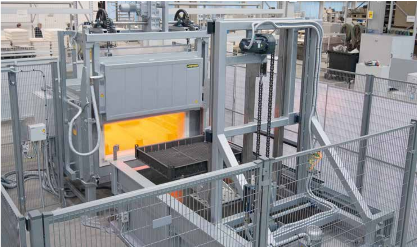
Automatic quenching and tempering plant N 644/S
