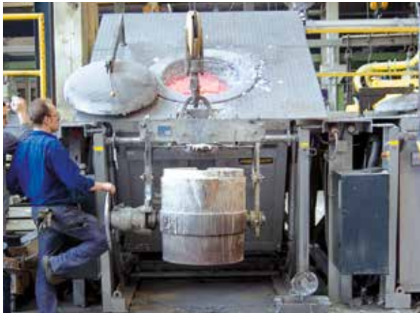
Charging of transport ladle with tilting furnace K 360/12
