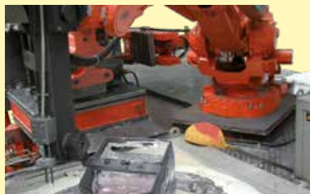
Bale-out of bale-out furnace with robot
