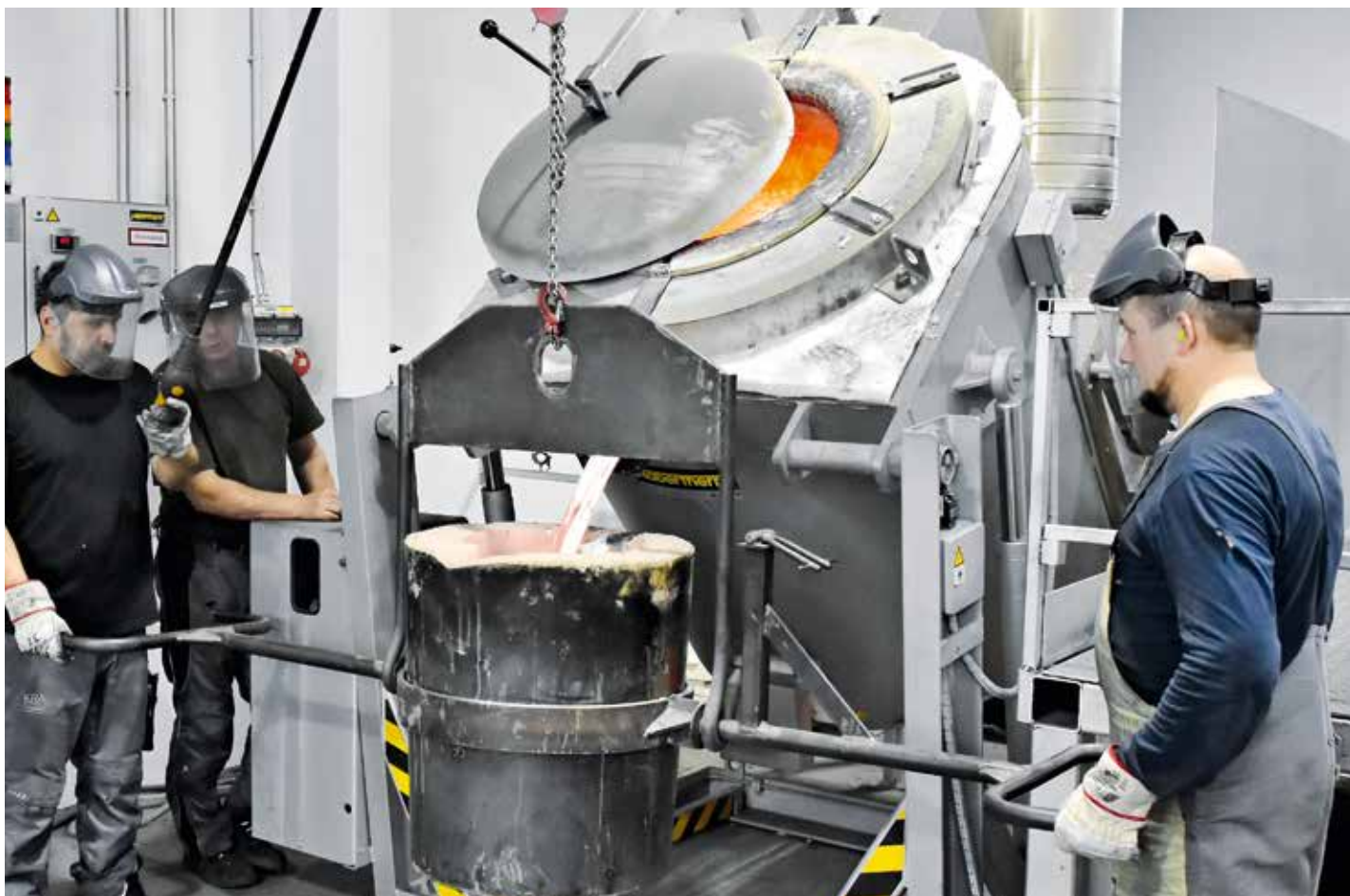
Tilting furnace KB 150/12 in production
