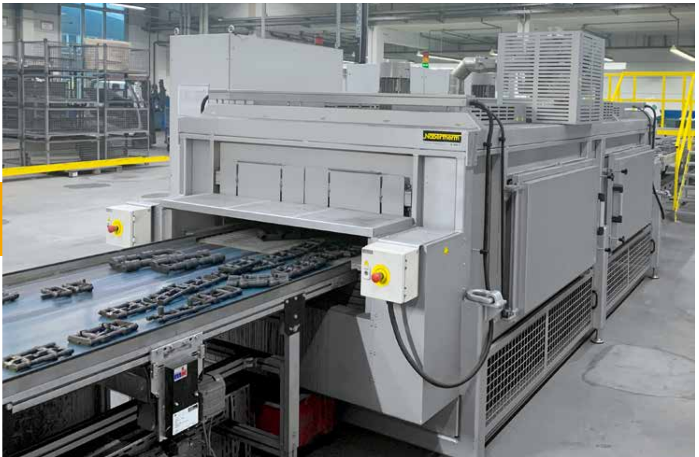
Continuous belt furnace D 1000/4000/140/35 AS for black wash drying on sand cores
