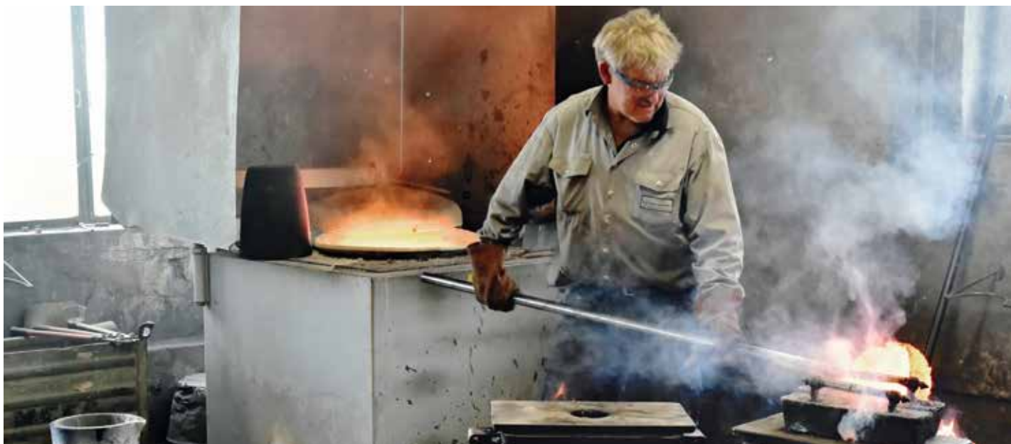
Bale-out furnace T 80/13 for gunmetal in a sand foundry shop
