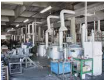
Recuperator burner for aluminum melting furnace 16 x TBR 110/12 and 2 x TBR 180/12
