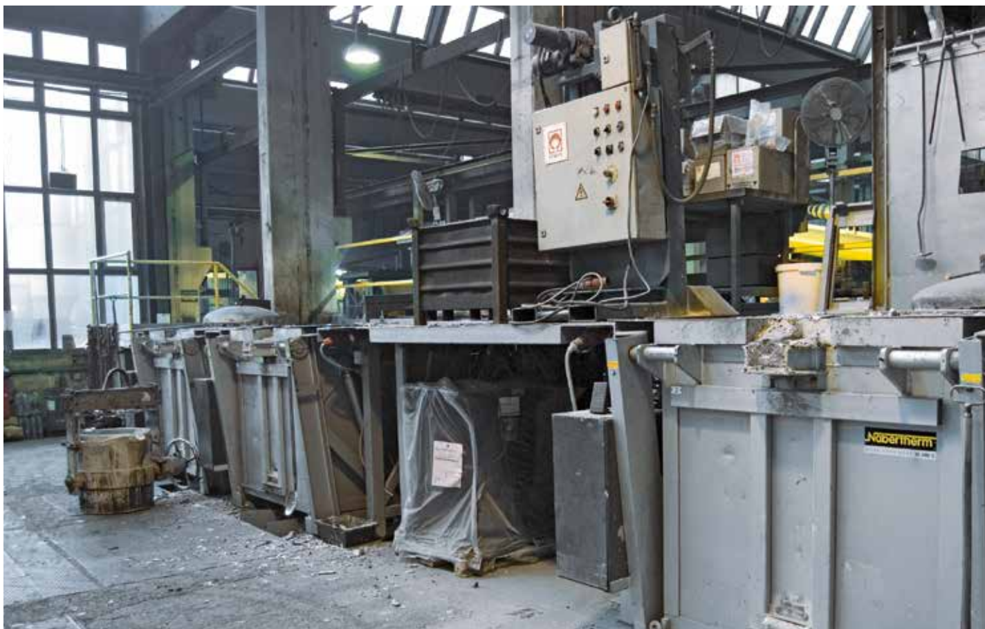
Three tilting furnaces with work platform for melting of aluminum
