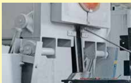
Tilting furnace K 40/13 with extended spout (sculpture foundry Knaak)
