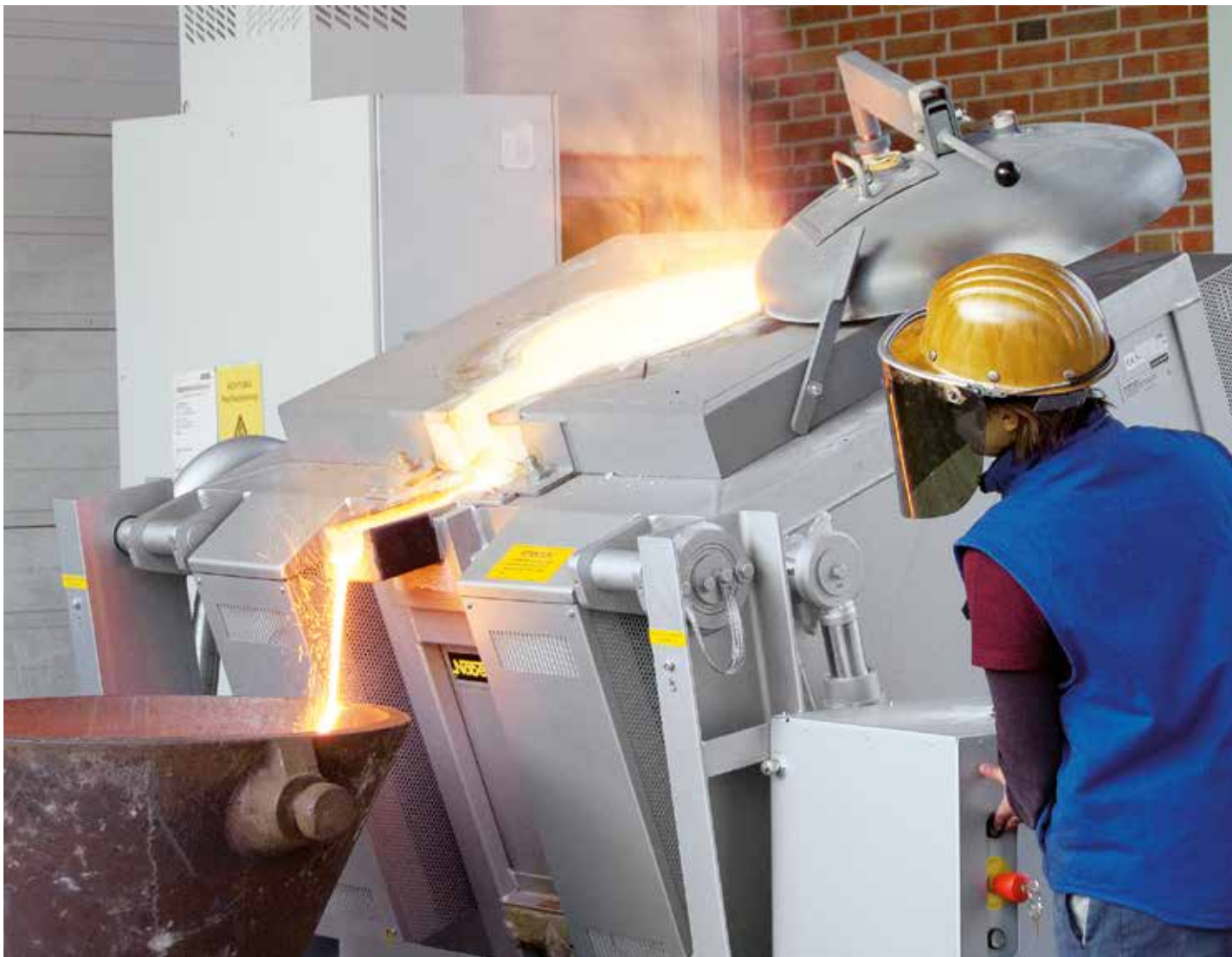
Tilting furnace KC 80/14 during casting
