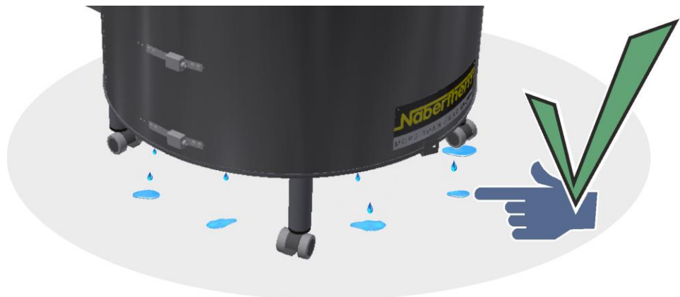
Fig. 26: Condensation accumulations during the first firings (similar to picture)
