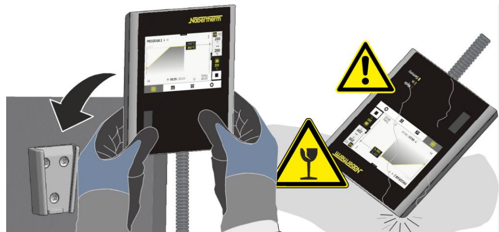
Fig. 30: Place the controller in the holder on the furnace (similar to the picture)
